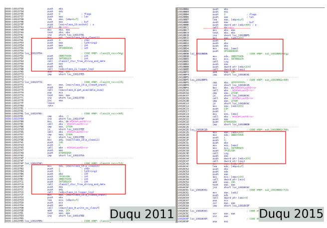
Another networking routine: after calling recv() to receive data from network, Duqu logs the results and possible network errors (obtained via WSAGetLastError()). Unique numbers in red rectangles are used to identify the current state of the networking routine.
