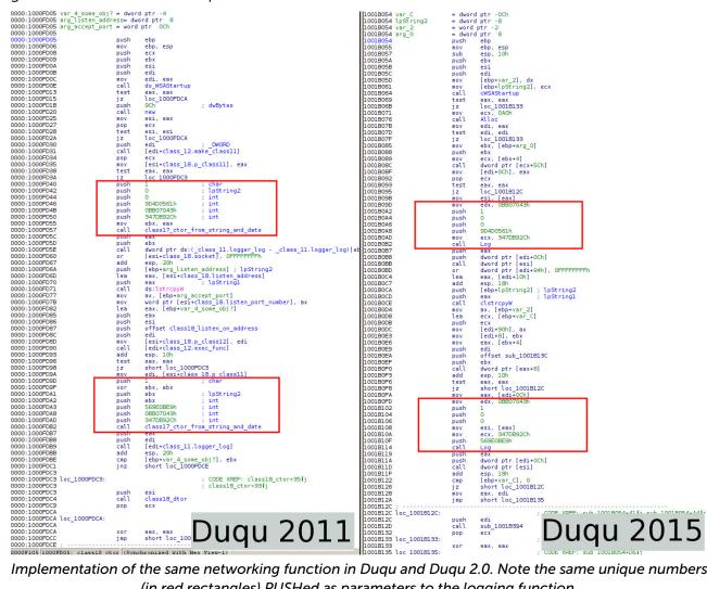
Implementation of the same networking function in Duqu and Duqu 2.0. Note the same unique numbers (in red rectangles) PUSHed as parameters to the logging function.
