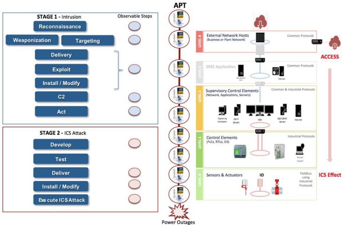
Figure 5: Ukraine Cyber Attack ICS Cyber Kill Chain and Purdue Model Mapping<sup>21</sup>
