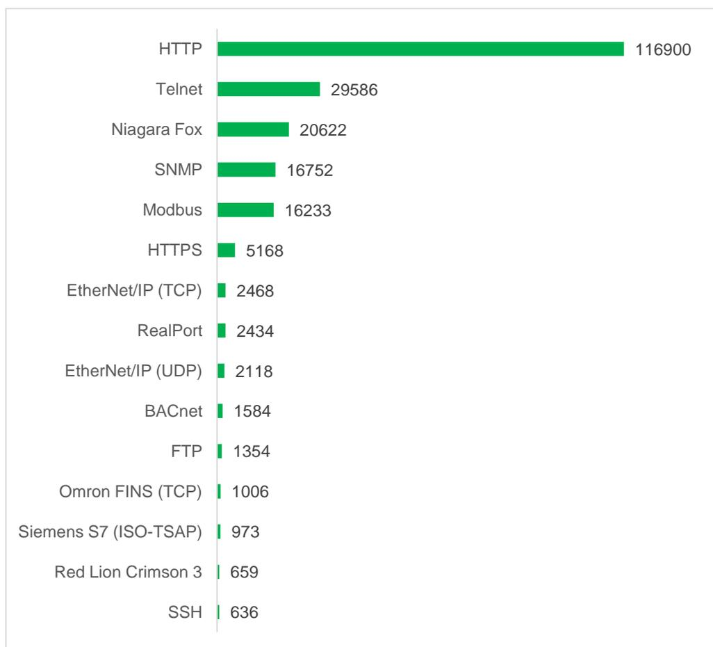
Figure 3. Top 15 protocols used by externally available ICS components
