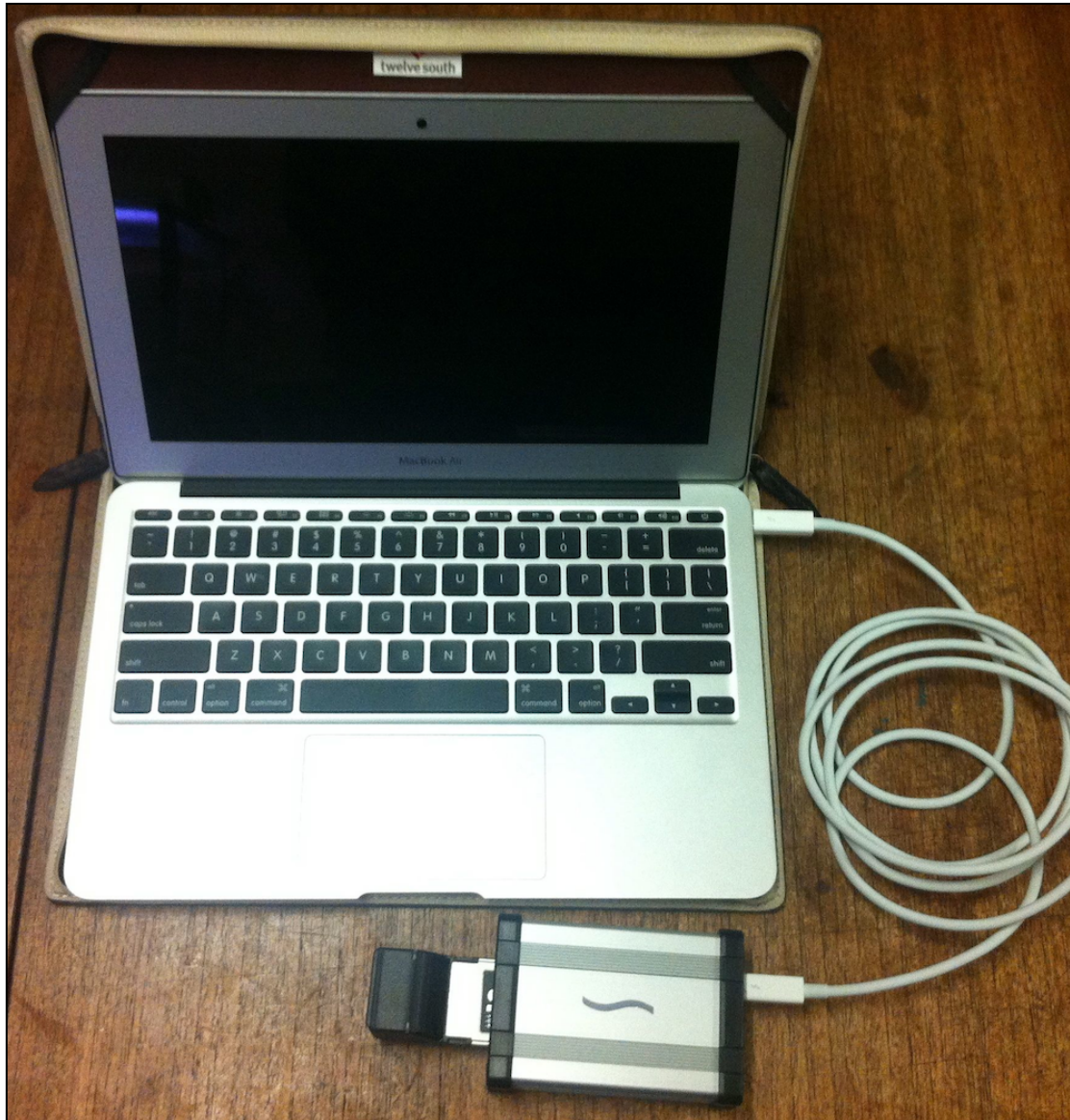
The first incarnation of the “evil maid” attack apparatus.
