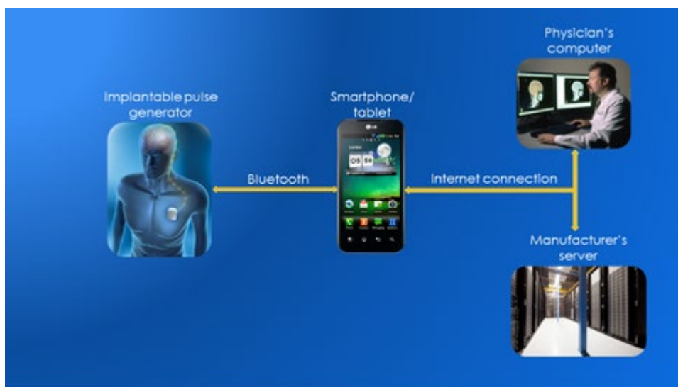
Fig: 1.0 - The connected architecture of implantable pulse generators. Source: University of Oxford, Functional Neurosurgery Group
