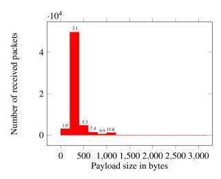
Figure 5: Histogram of the payload size from the DHT responses which are caused by get\_peers requests. The numbers on top of the bars are the average BAF values.
