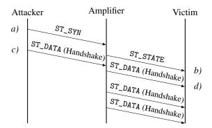
Figure 3: In uTP the initiator sends a ST\_SYN packet to the receiver. The receiver acknowledgs this with a ST\_STATE packet. After that, the connection is established (two-way handshake).
