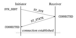
Figure 2: Two-way handshake to initiate a connection between two uTP nodes. The text on the outer edge reflects the state of the protocol.
